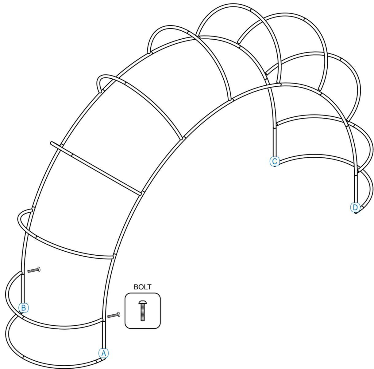
Snap all shock corded tubing together. Connect side rails to bottom rails. Align alphabetical labels. Bolt ribs between side rails.
